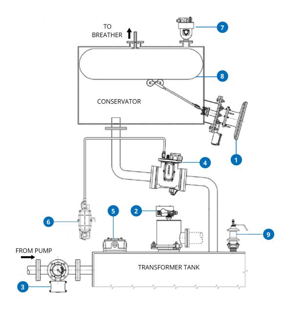
1 Oil Level Indicator 2 Pressure Relief Valve 3 Flow Indicator 4 Buchholz Relay
